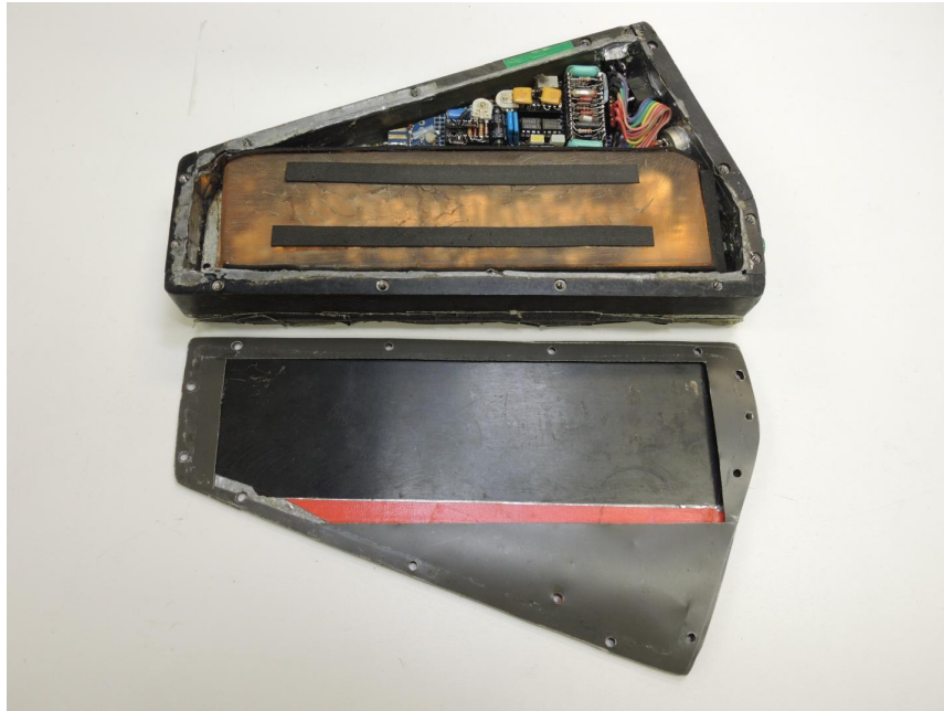
Figure 3. Early Mu-metal shielded Apocalypse Now Beam pickup, mid 1980s
