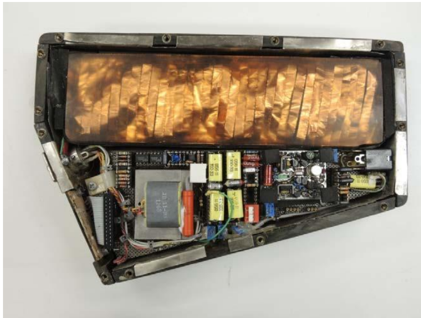
Figure 4. Single-coil Beam pickup design with early discrete component electronics, late 1980s
